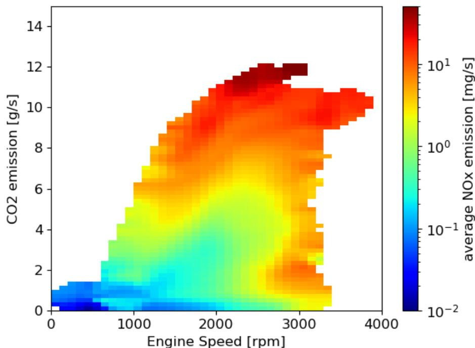
Figure 1 Example emission map of test vehicle
